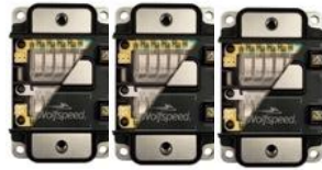
Lucid Traction Inverter with 3 10-die modules
