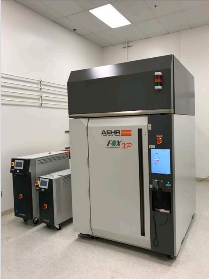
FOX-XP 18 Wafer SiC Test & Burn-In System configured for SiC Gate Stress Test
