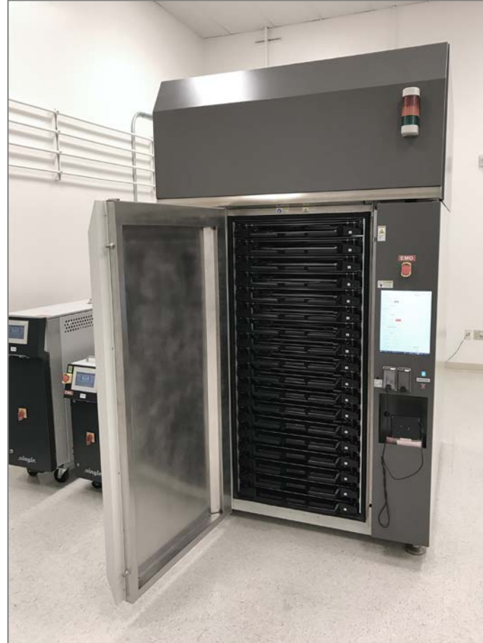
FOX-XP 18 Wafer SiC Test & Burn-In System configured for SiC Gate Stress Test
