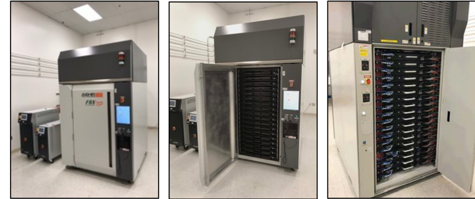
FOX-XP 18 Wafer Test & Burn-In System
