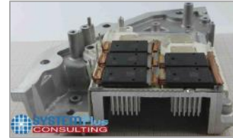
Tesla Model 3 Inverter with ST SiC Power Modules
