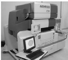
The FOX™-1 Full Wafer Parallel Test System is designed to make contact with all die on an IC wafer simultaneously, thus enabling high-throughput massively parallel test of the entire wafer at one time. Since the FOX-1 system can electrically test all of the die on a wafer in a single touchdown, we believe it will significantly reduce the cost of testing wafers.
