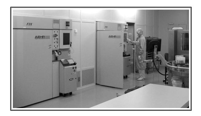
Aehr Test Systems FOX-15 Wafer-Level Test and Burn-In System Installation
