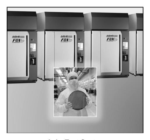
Aehr Test Systems FOX-XP Multi-Wafer Test Systems
