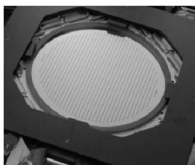
WaferPak™ Cartridges interface from the FOX-1 or FOX-15 system to the customer's wafer to be tested or burned-in. They contain micro-miniature probes to contact all of the die on a wafer in a single touchdown. WaferPak Cartridges are custom designed uniquely for each customer wafer application to interface to the unique pad positions of a wafer design. When used in a FOX system, WaferPak Cartridges enable the production of Known-Good Die (KGD) for use in multi-chip packages.
